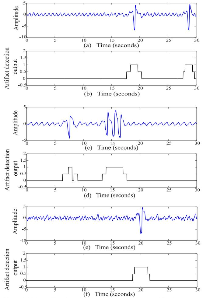
Figure 4. Noise artifact detection algorithm output for several PPG segments: (a)–(d) normal sinus rhythm; (e)–(f) AF segment.
