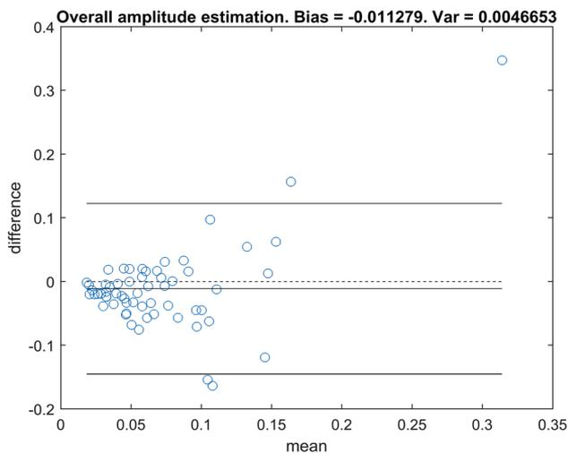
**FIGURE 6. Bland–Altman plot for comparison of amplitude measures using Ag/AgCl and CB/PDMS electrodes. Bias = - 11.3  $\mu$ V, variance =  $4.6 \times 10^{-3}$ .**
