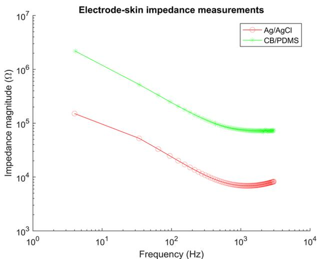
FIGURE 4. Electrode-skin contact impedance measurements for Ag/AgCl and CB/PDMS electrodes.
