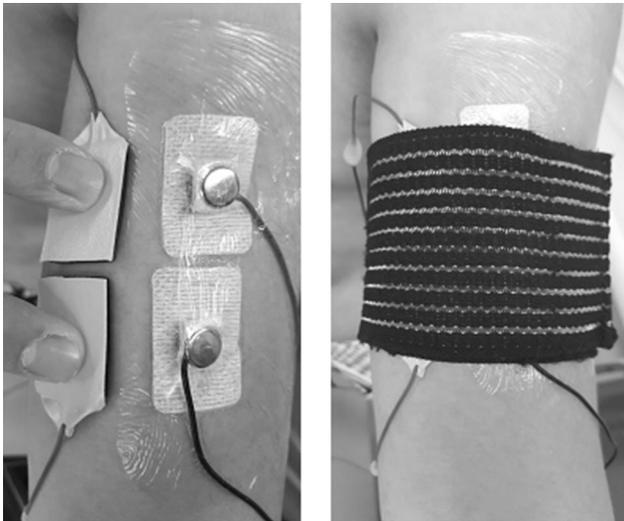
**FIGURE 1.** Left: CB/PDMS and Ag/AgCl electrodes on a subject's biceps. Notice that Ag/AgCl electrodes shown on the right side of the left figure are waterproofed with Tegaderm<sup>®</sup>. Right: Velcro strap to keep electrodes in place.
