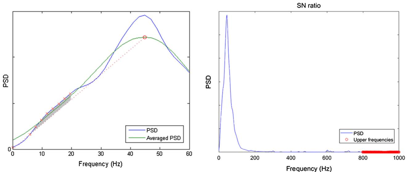
FIGURE 3. Illustration of SM ratio (left) and SN ratio (right) estimation.
