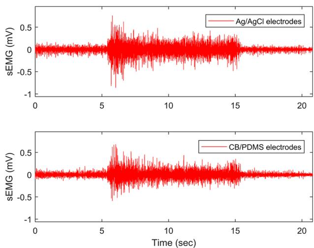
FIGURE 5. sEMG signal acquired under water using Ag/AgCl (top) and CB/PDMS electrodes (bottom), for a given subject’s biceps.
