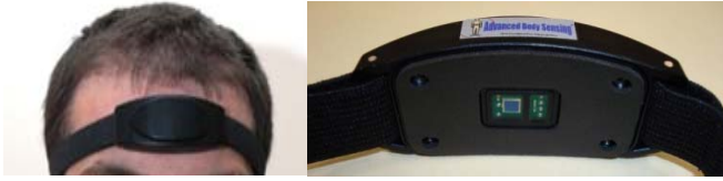
Fig. 1. Dual-wavelength forehead wearable pulse oximeter.
