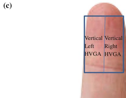
Division of Camera's Field of View into Vertical Left Half VGA & Right Half VGA
