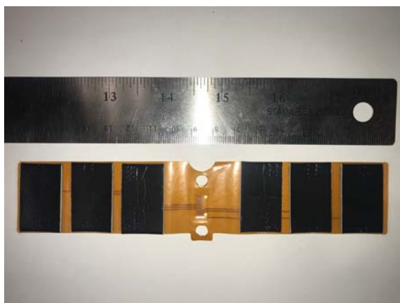
Fig. 1. a) Armband device prototype and electrode configuration for the 3 ECG channels and the EMG channel. b) Sensing part of the prototype.
