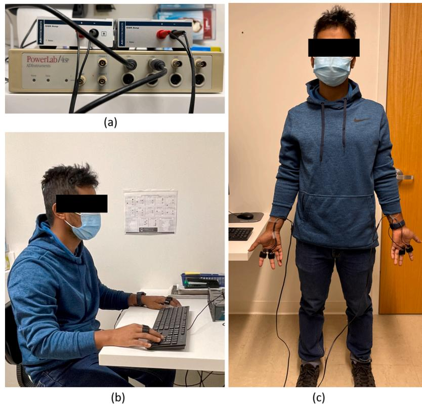
**Fig. 2.** Data collection: (a) ADInstrument PowerLab and GSR module (b) Subject typing with one hand (c) Subject wearing electrodes on both hands.
